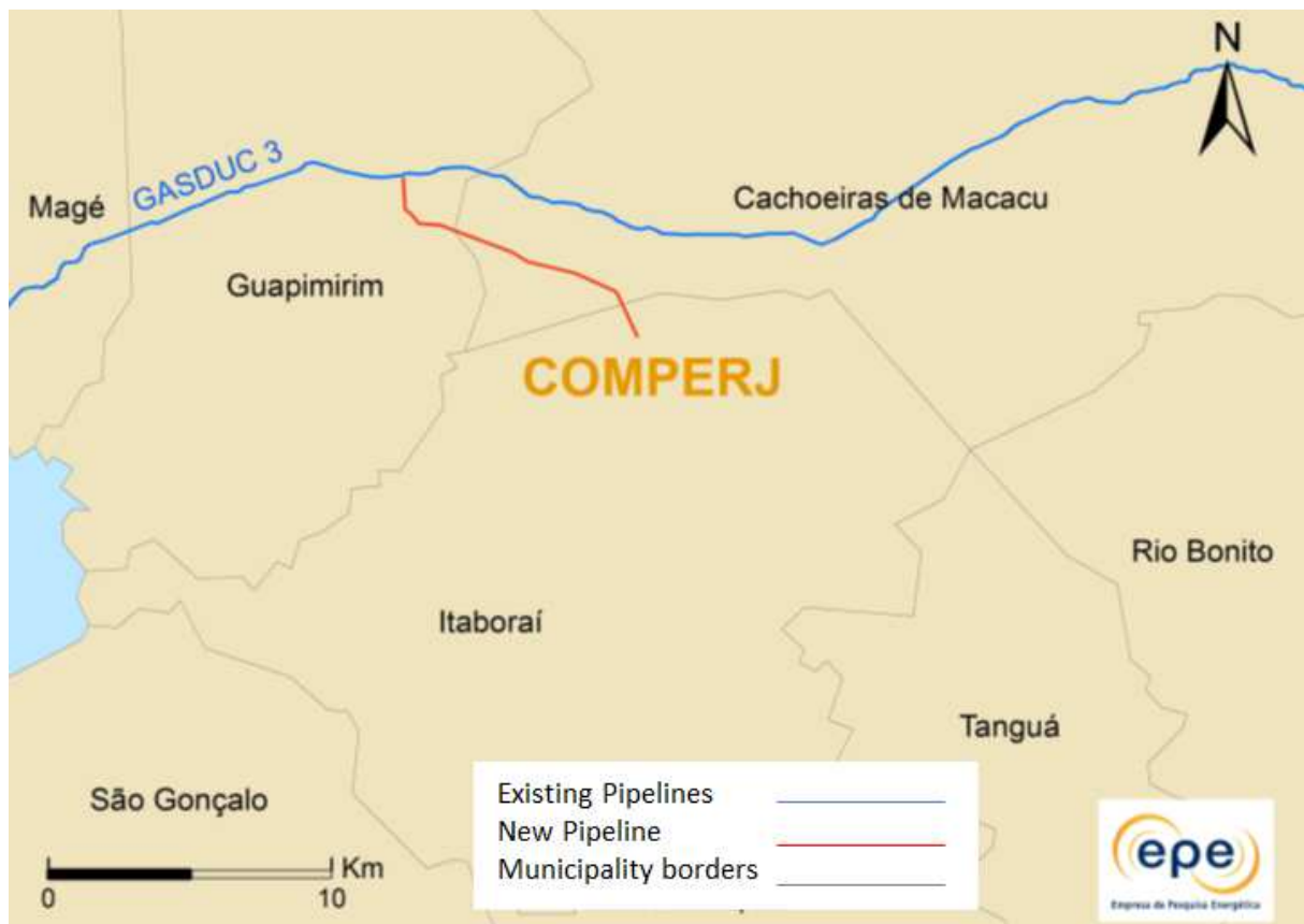
Figure 2.38 COMPERJ, Itaboraí/RJ – Southwest Integrated Network/RJ – Preliminary Proposed Route
