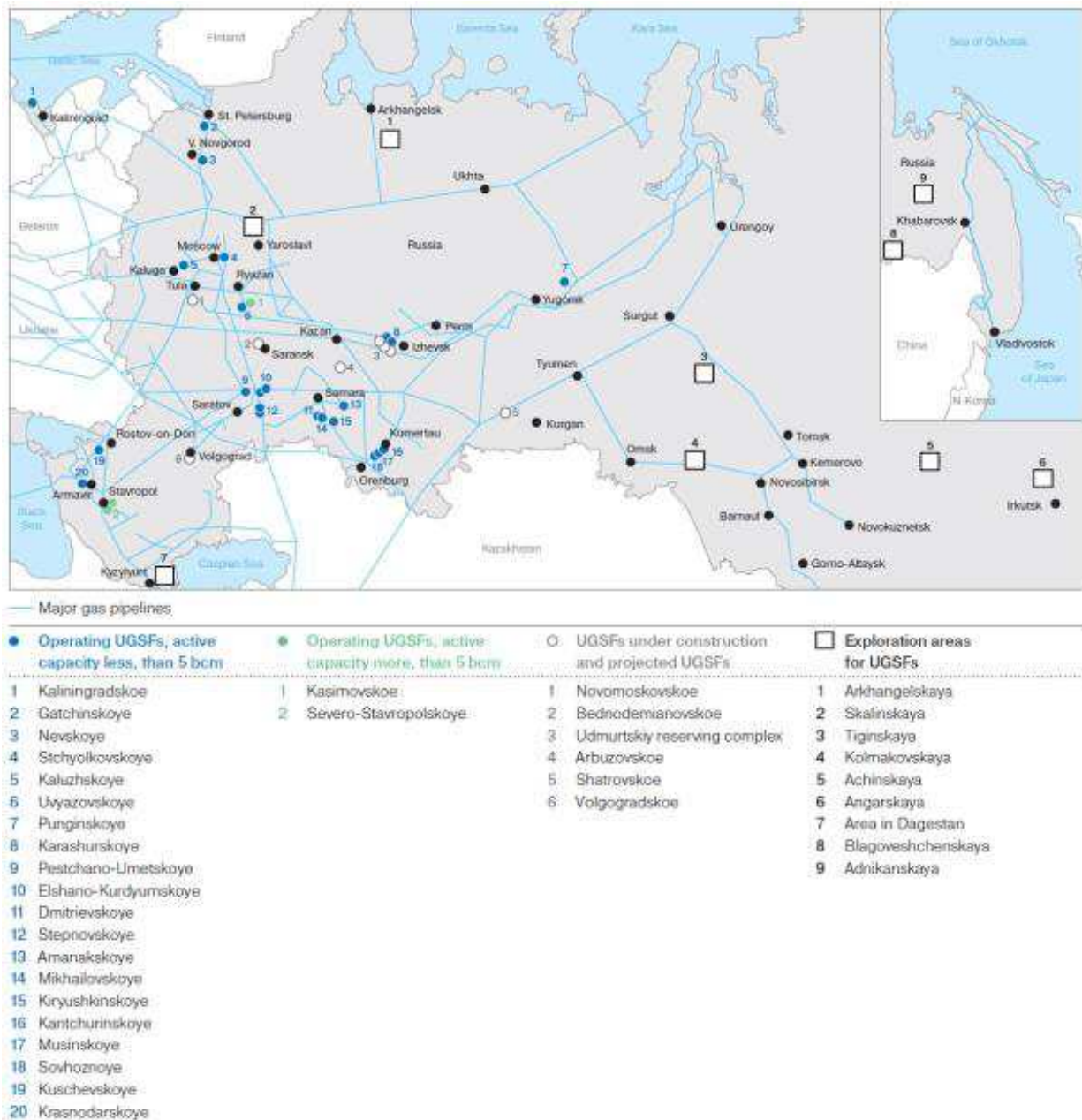
Figure 2.21 Gazprom's operational and prospective UGS facilities in Russia (source: Gazprom)
