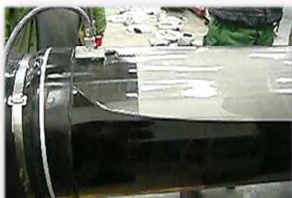
Leakage test Shell made of transparent material
