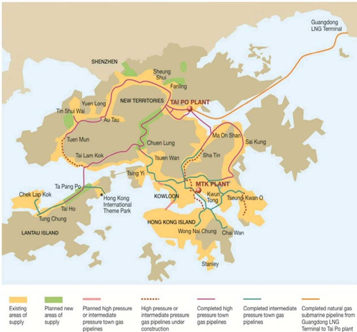
Figure 2.30 Towngas distribution gas network in Hong Kong comprising 3,500 km of natural gas pipelines
