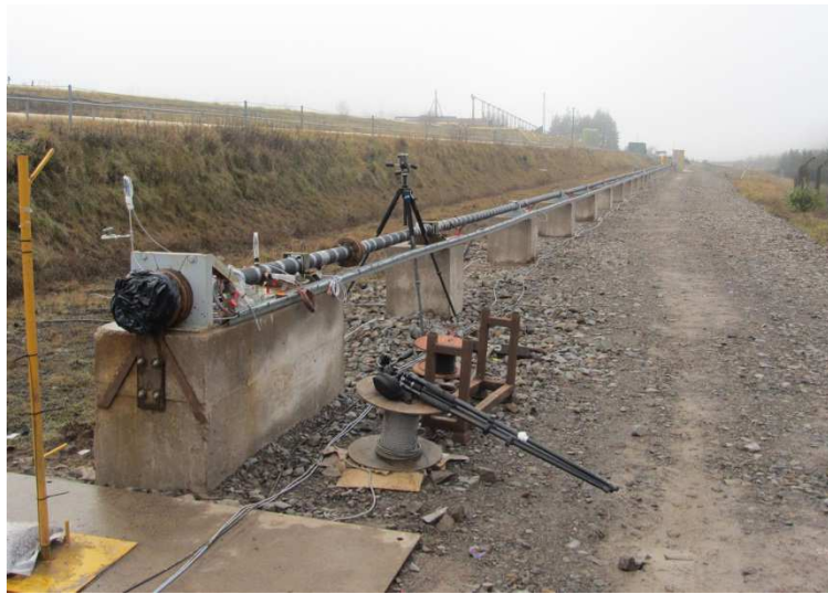
Figure 8.5 Depressurisation rig at Spadeadam GL Noble Denton
