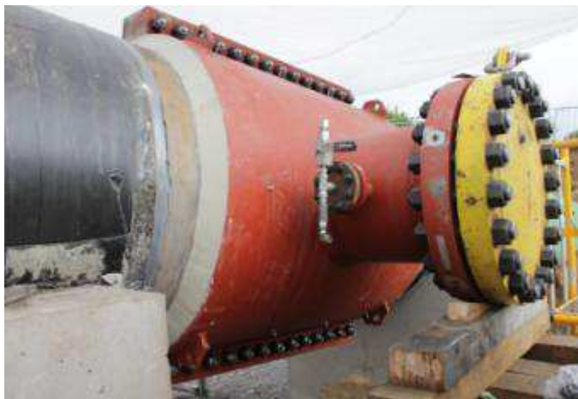
Figure 6.37 42" x 18" Class 600 grouted tee
