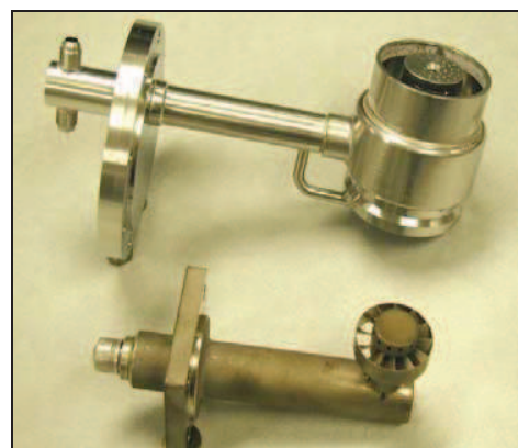
Figure 10a. Comparison of Taurus 60 SoLoNOx and Conventional Combustion System Fuel Injectors
