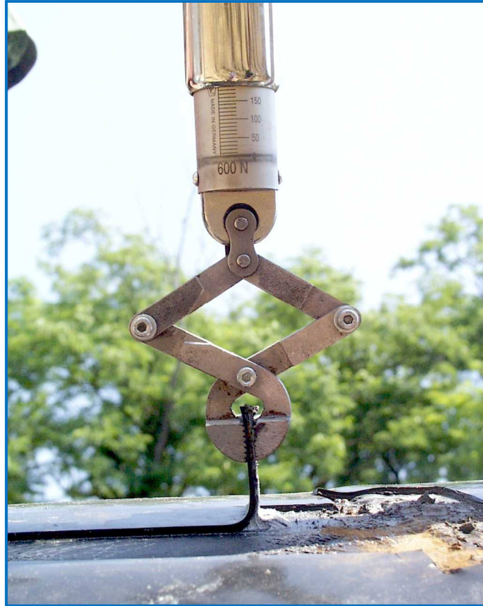
Figure 6.47 Tear test of the rehab shrink cuff
